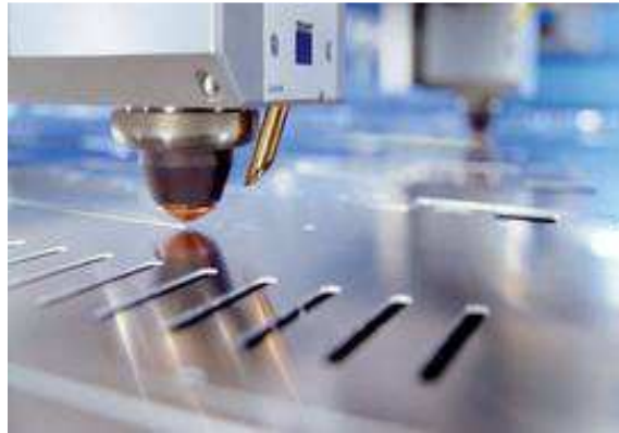
Figure 2: Melting, Burning, Evaporating, Blowing - and Still the Human Eye Only Sees a Cutting Head Moving over the Sheet Metal [2]
