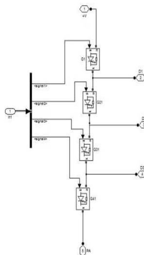
**Figure 3: Subsystem of Five Level Inverter**
