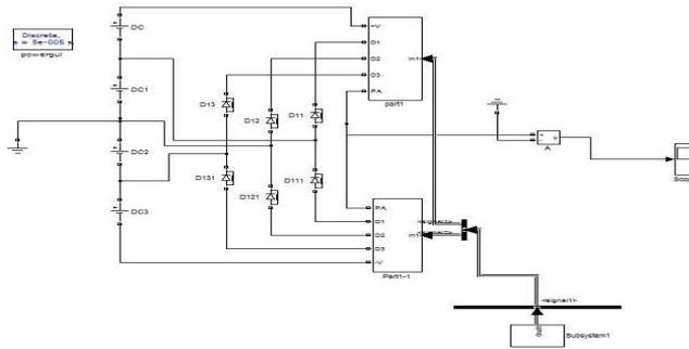
Figure 2: Five Level Converter
