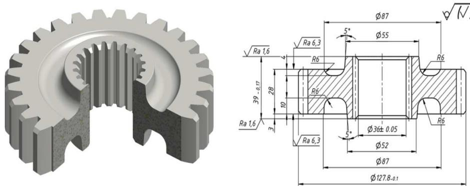
**Figure 2: 3D Model and Drawing Details (Gear)**
