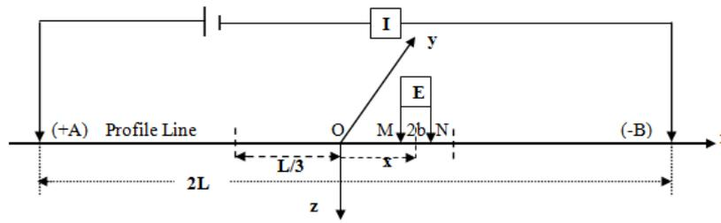
**Figure 2: Field Lay-Out of Gradient Profiling Where A, B = Current Electrodes with  $2L$  Distance and M, N = Potential Electrodes with  $2b$  Distance,  $I$  = Current Supplied in the Earth and E, the Measured Electric Field =  $\Delta V/2b$**
