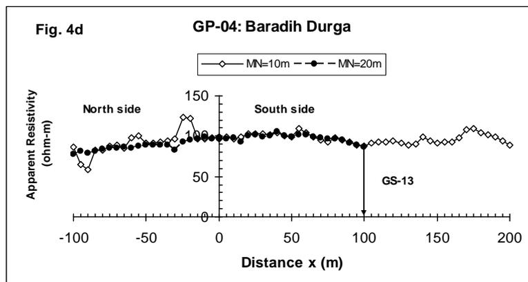
Figure 4D: Showing the Apparent Resistivity Response along Profile GP-04 (Baradih Durga) Covering 300 M Length for MN=10 M and MN=20 M and Position of One Selected Location GS-13 on the Profile
