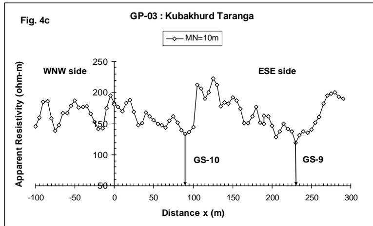
Figure 4C: Showing the Apparent Resistivity Response Along Profile GP-03 (Kubakhurd Taranga) Covering 400 M Length for MN=10 M and Position of Two Selected Locations GS-09 and GS-10 on the Profile
