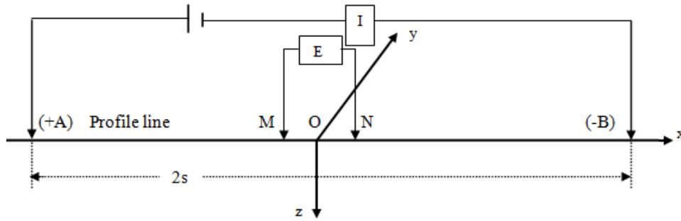
Figure 3: Lay-Out of Schlumberger Configuration.
