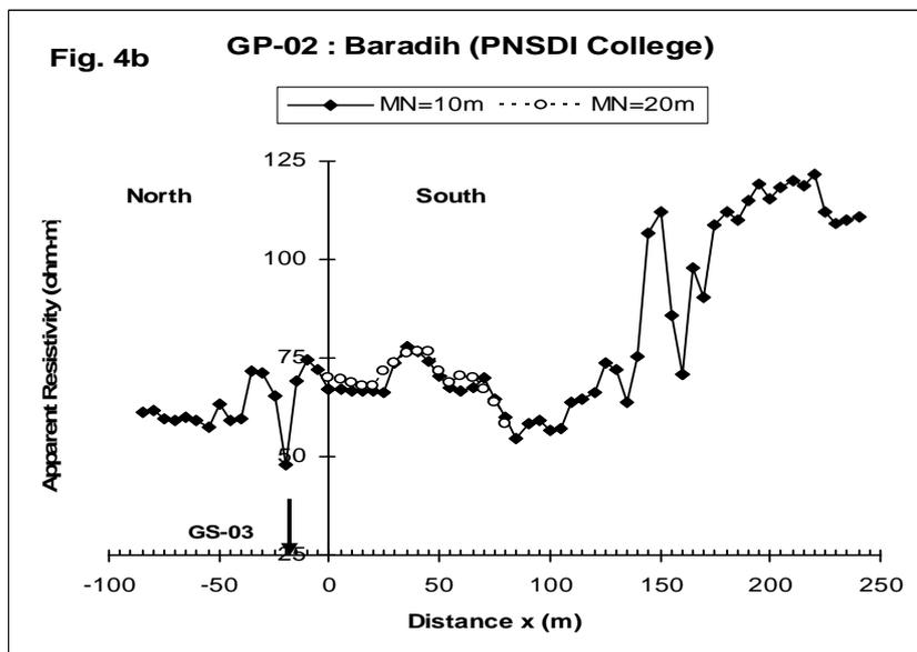
Figure 4B: Showing the Apparent Resistivity Response along Profile GP-02 (Baradih -PNSDI College) Covering 350 M Length for MN=10 M and 20 M and Position of One Selected Location GS-03 on the Profile
