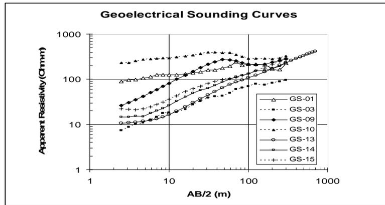
Figure (5): Showing the Apparent Resistivity Response of Goelectrical Soundings Obtained at Various Locations with Varying Current Electrode Separation, AB/2
