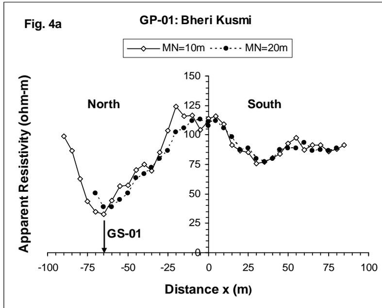
Figure 4(a): Showing the Apparent Resistivity Response along Profile GP-01 (Bheri Kusmi) Covering 200 M Length for MN=10 M and 20 M and Position of One Selected Location GS-01 on the Profile
