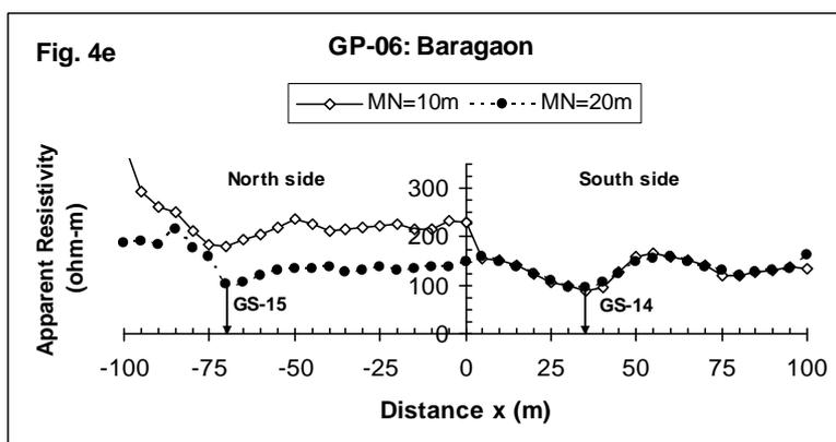
Figure 4E: Showing the Apparent Resistivity Response along Profile GP-06 (Baragaon) Covering 200 M Length for MN=10 M and MN=20 M and Position of Two Selected Locations GS-14 and GS-15 on the Profile
